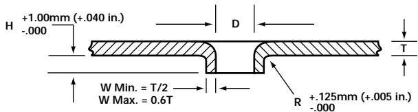
Extruding holes for fasteners in light-gauge steel nearly doubles the length of thread engagement over original material thickness.
