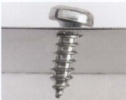
Standard type AB screws lean over as the screw tends to align with the helix angle of the thread. Stripped threads or loose assemblies result.
