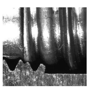
The lead thread of the externally threaded (male) member engages into an underfilled internal female thread (a.k.a. crest-crater)
