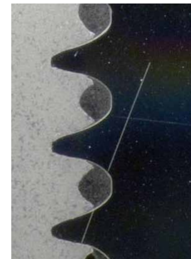
Metallographic cut of the play-free engagement between male and formed female thread
