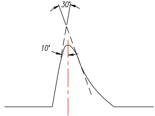
The REMFORM® II™ "F" asymmetrical Unique Radius Flank™ thread form has the thread-forming advantages of a 30° thread, without the difficulty of manufacturing a 30° thread.
