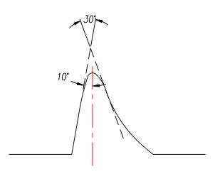
The REMFORM® II $^{\text{TM}}$  "HS" unique asymmetrical radius flank thread form has the thread forming advantages of a 30° thread, without the difficulty of manufacturing a 30° thread.
