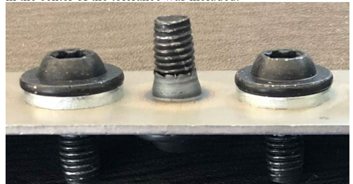
FIGURE 10: FLOW DRILLED HOLES IN 1.1MM THICK GEN 3 1200MPa STEEL WITH AN M5 RHS SCREW DRIVEN THROUGH THE FLOW DRILLED HOLE
