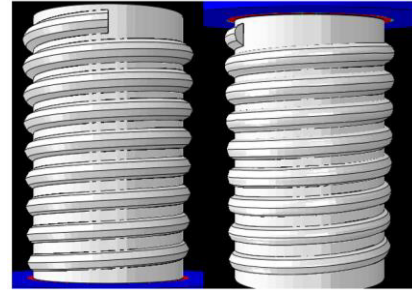
FIGURE 9: RHS SIMULATED THREAD SHAPE BEFORE AND AFTER THREADFORMING IN 3MM THICK HSLA550
