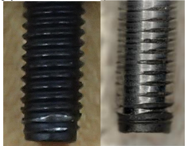
FIGURE 4: (LEFT) DAMAGED LEAD THREADS ON TRIROUNDULAR PART AFTER IT WAS DRIVEN IN HSLA550, THIS PART STALLED DUE TO THE THREAD DAMAGE. (RIGHT) FULL DAMAGED THREADS FROM FORCING THE TRIROUNDULAR SCREW TO DRIVE EVEN WITH LEAD THREAD DAMAGE (LARGE DOWNFORCE).
