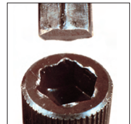
Tool and fastener damage is common
