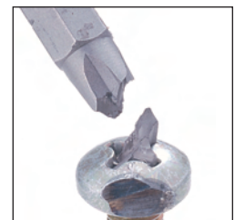
Concentrated stresses can cause breakage
